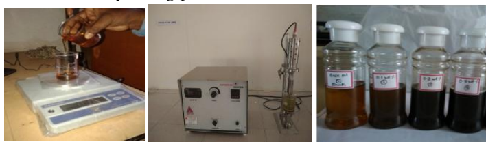
Fig. 2: Weighing and Probe sonication of CuO-Engine oils.
