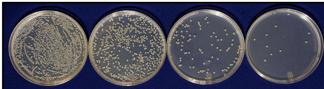
Agar plating method for viable cell counts using dilutions 1 \times 10^5 , 1 \times 10^6 , 1 \times 10^7 , and 1 \times 10^8
