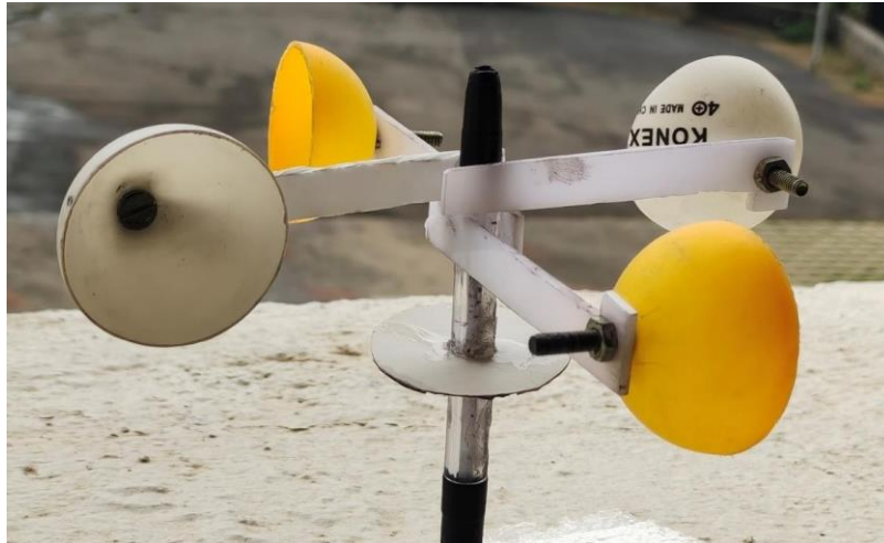
Fig. 2: A 4-cup anemometer
