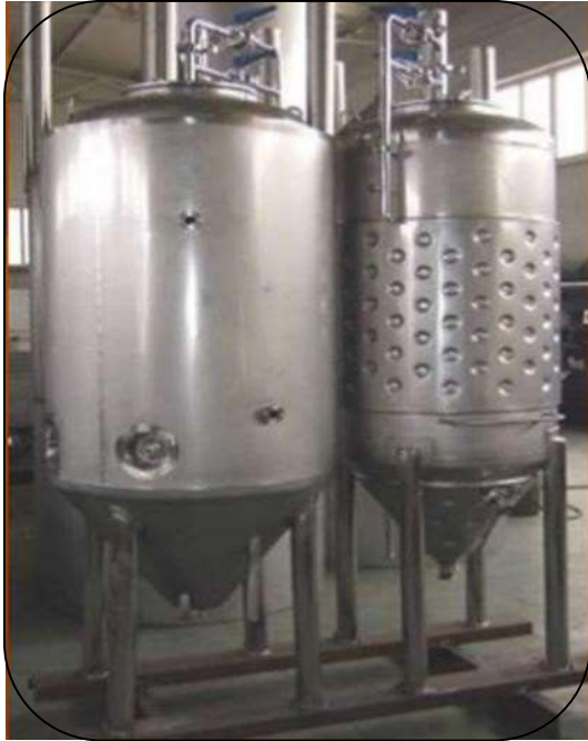
Plate 1 (a): Yeast propagation in propagating vessels
