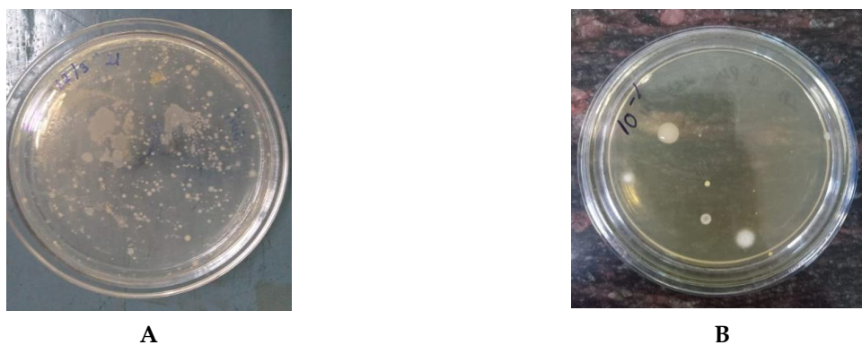
Fig. 4: Untreated water microbial count (A), Treated water count (B)
