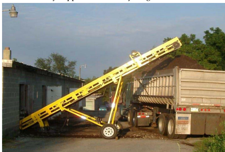
Fig. 8: Post-crop mushroom compost (MC) being loaded onto a truck as it is removed from a mushroom house
