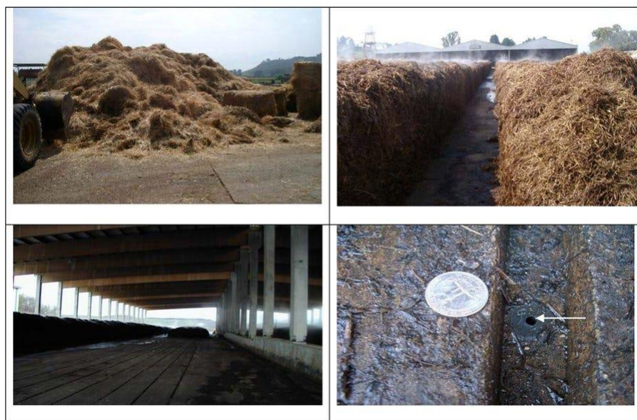
Fig. 1: Loose straw ready for incorporation into compost windrow (top left); compost windrow (top right); aerated Phase I compost wharf under roof (note groves in concrete, bottom left); groove showing aeration nozzle (bottom right, arrow)
