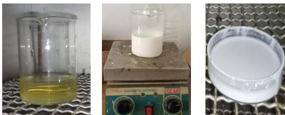
Fig. 2: Culture Supernatant (A), ZnO added to culture supernatant (B) ZnO nanoparticles Collected and dried (C)
