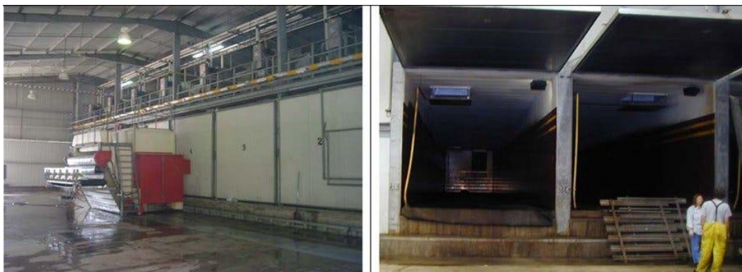
Fig. 2: Phase II tunnels used to pasteurize and condition compost for mushroom production. Left: filling machine in front of closed tunnel, Right: open tunnel ready for filling
