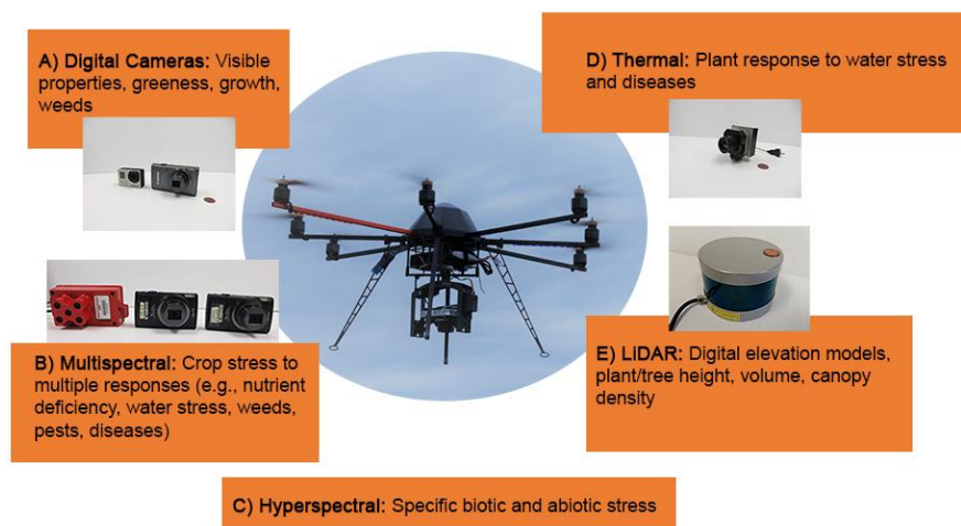
Fig. 3: Sensors integrated with Drone (Khot, 2017)
