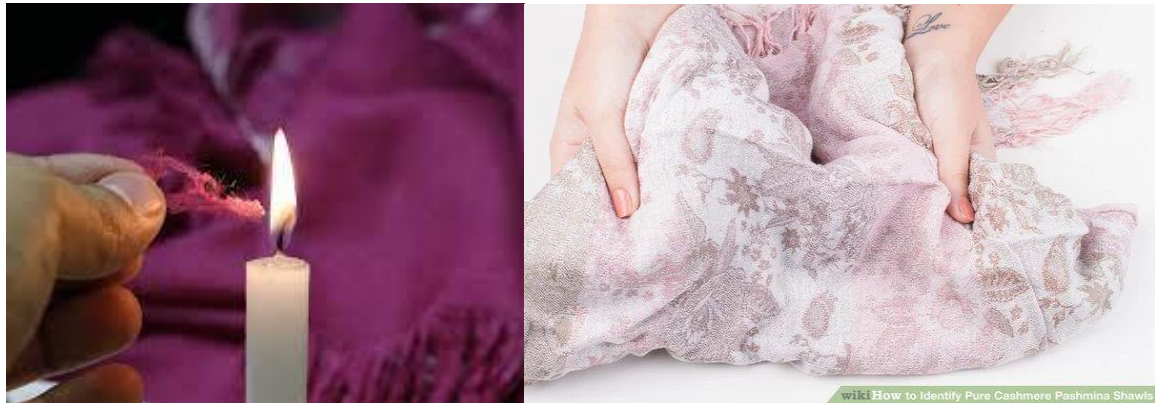
Figure 7: Burning and Rubbing test of Pashmina fibre produced by Changthangi goat
