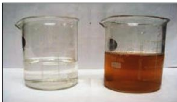
Figure 2: Synthesis of silver nanoparticles using BPE
