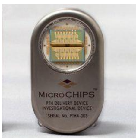
Figure 3: Implantable drug-releasing micro-chips
