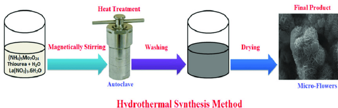
Fig. 7 : Schematic diagram of hydrothermal synthesis process for 3D flower
