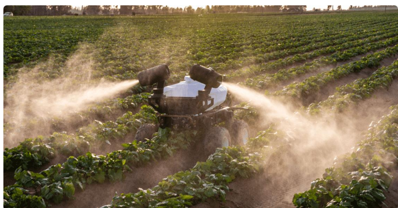
Fig. 3: Use of UGV for precision application of chemicals
