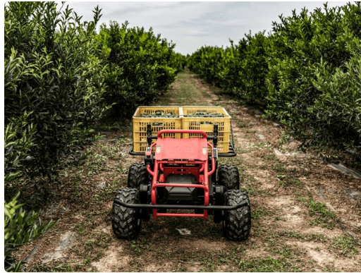
Fig. 4: UGV used for transportation work in the orchard ( https://www.xa.com/en/r150 )
