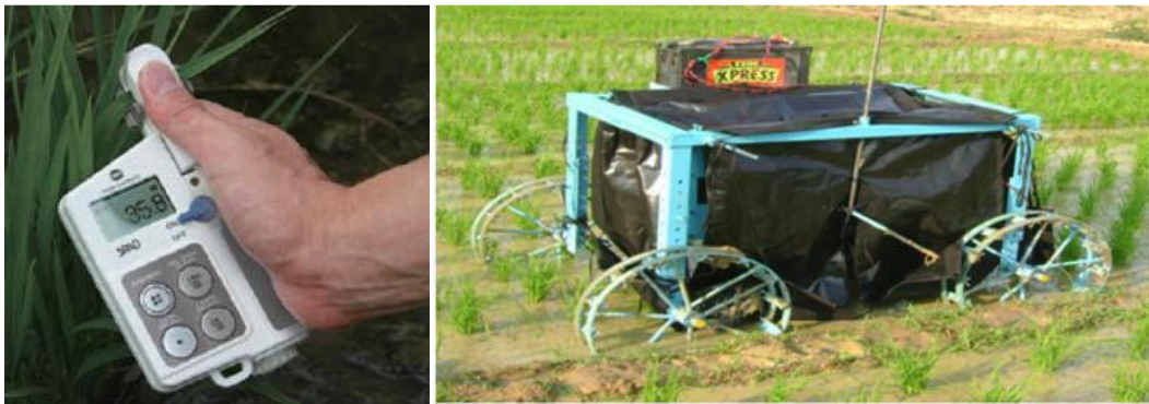
Fig. 8a: SPAD metre and colour sensor for capturing the plant image in paddy field
