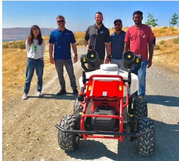
Fig. 2: UGV for precision application of agrochemicals
