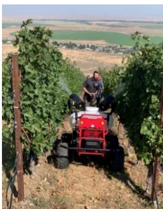
Fig. 3: Use of UGV for precision application of chemicals
