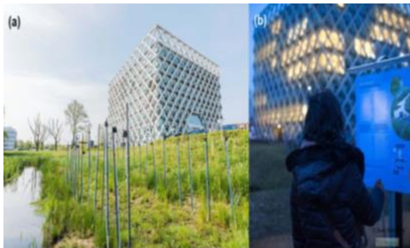
Figure 9: (a) A tubular PMFC system for demonstration purposes at the Wageningen campus. (b) Visitors can press the button to turn on the LED light powered by the PMFC system (Plant-e, 2016).
