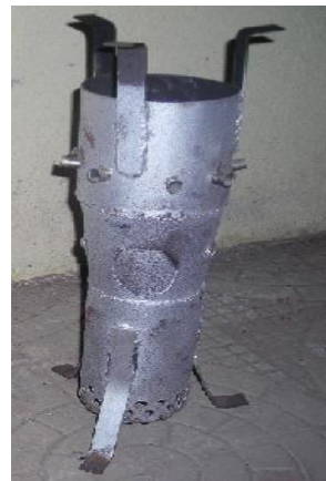
Fig 2: Photograph of Micro-Gasifier
