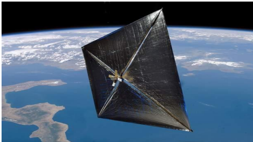
Fig. 2: The Solar Sail Demonstration mission led by NASA and L'Garde Inc. aimed to prove the viability of using ultra thin sails and sunlight for propulsion (Image courtesy of NASA)
