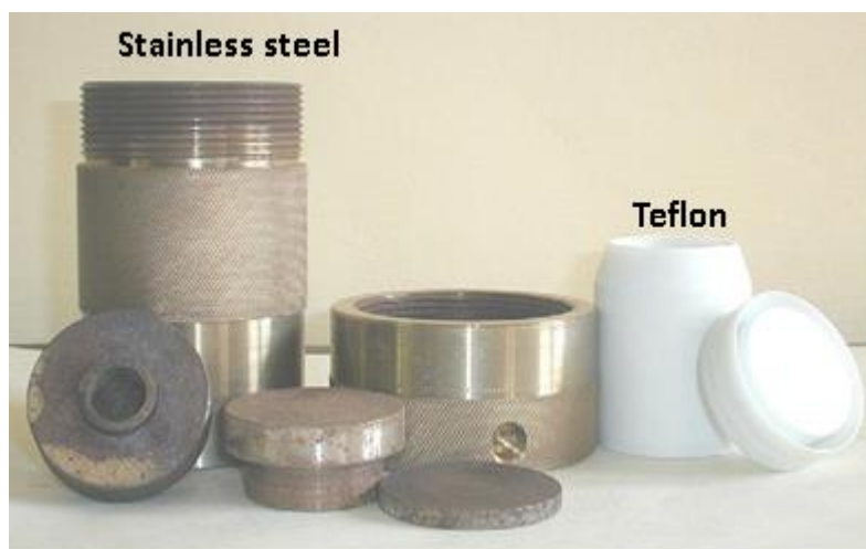
Fig. 1.7: Autoclave with Teflon cylinder used for hydrothermal synthesis
