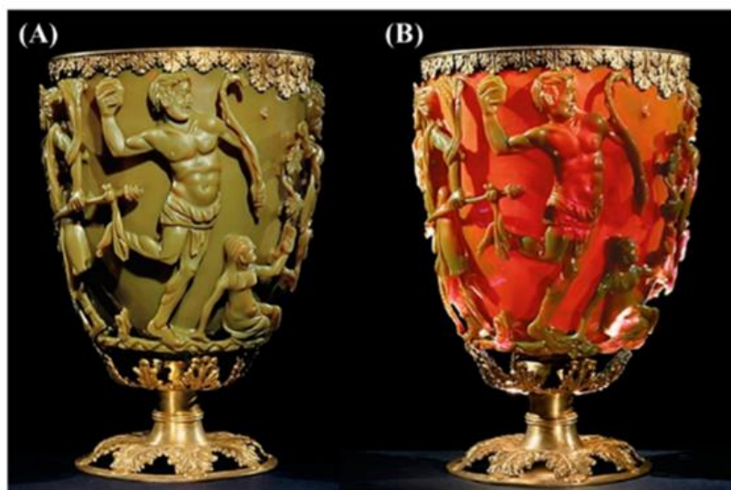
Fig. 2: Lycurgus vessel. The glass appears green in reflected light (A) and red-violet in transmitted light (B)
