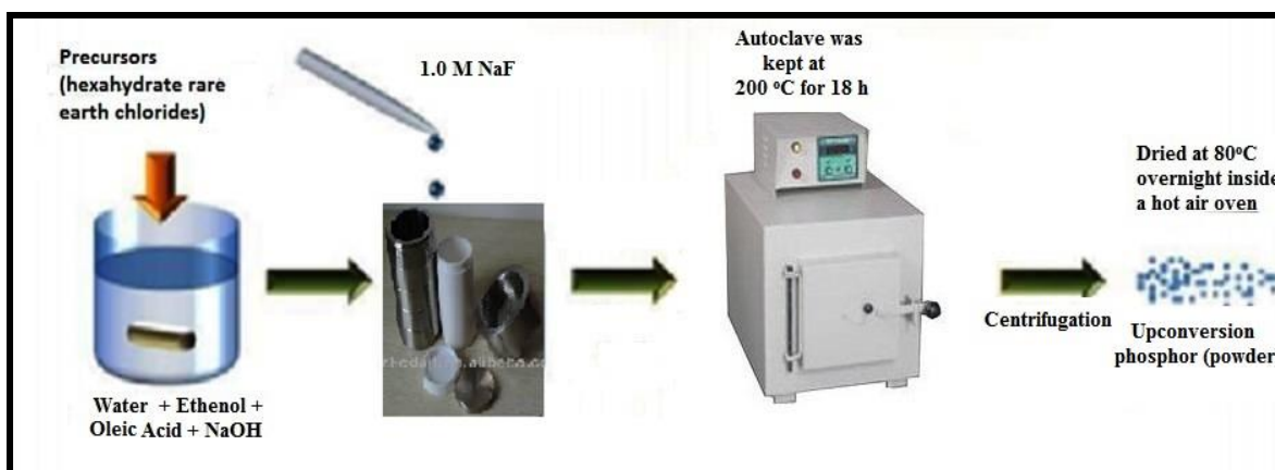
Figure 3: Schematic diagram shows the set up of synthesizing hydrothermal assisted NaYF 4 : Yb 3+ /Er 3+ upconversion phosphor materials
