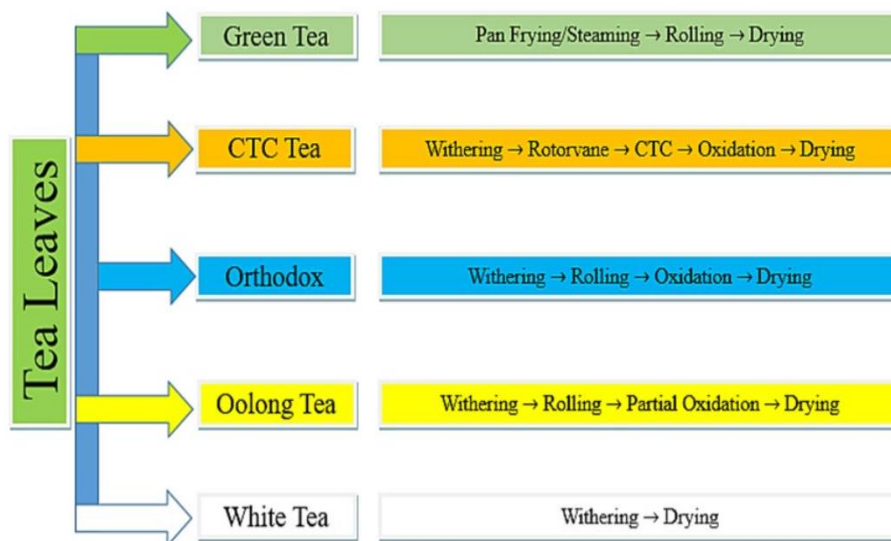
Figure 3: Steps involved in production of various varieties of tea ((Aditya et al. , 2023)
