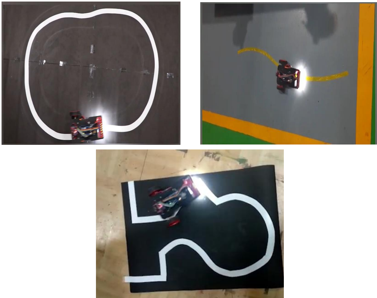
Fig. 5: Results Obtained from Line follower Robots mounted with Designed Light Sensor Module
